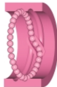
Fig 3.5 Circuit for internal return cap
