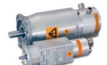
The EX Servo motors are designed to function in Category II, Group II explosive atmospheres in respect to the EN 50014 standard. These servo-motors are certified according to directive ATEX 94/9/CE and are available in a Gas or Gas-Dust version. The motors differ in that the Gas-Dust version is equipped with a special lip seal on the customer end shaft.
